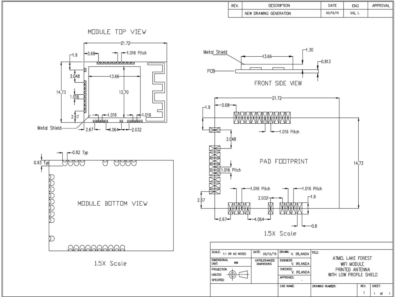
Figure 3-3. Module Drawings – WINC1500-MR210UB - Top and Bottom Views (unit = mm)
